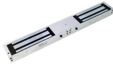
The DS-K4H450D double-door magnetic lock is designed for wooden door, glass door, metal door, and fireproof door. The maximum thrust of the lock is 500 kg (1102.5 lbs) × 2. It can be used for controlling door opening/closing, and the indicator shows the door status. It supports signal output of door lock output status testing.
