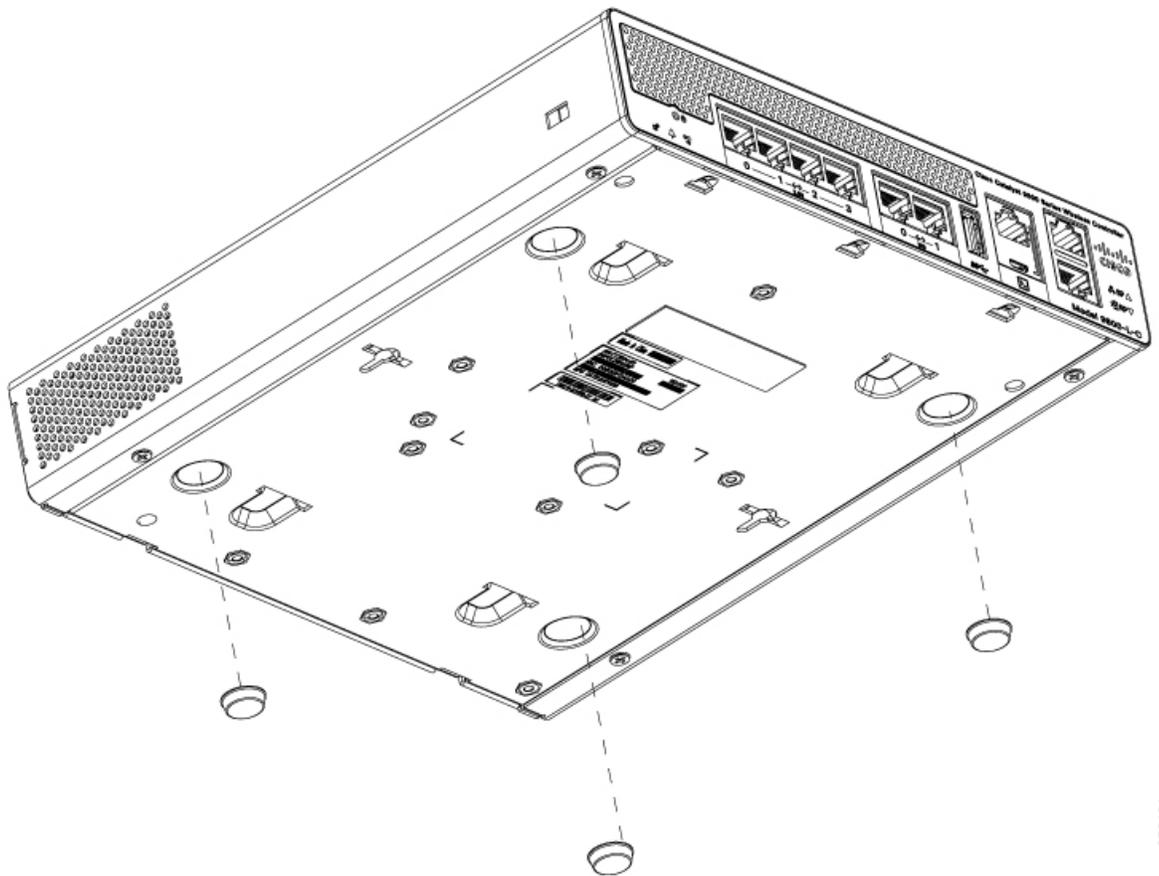
**Step 4** Place the controller right-side up on a flat, smooth, secure surface.
