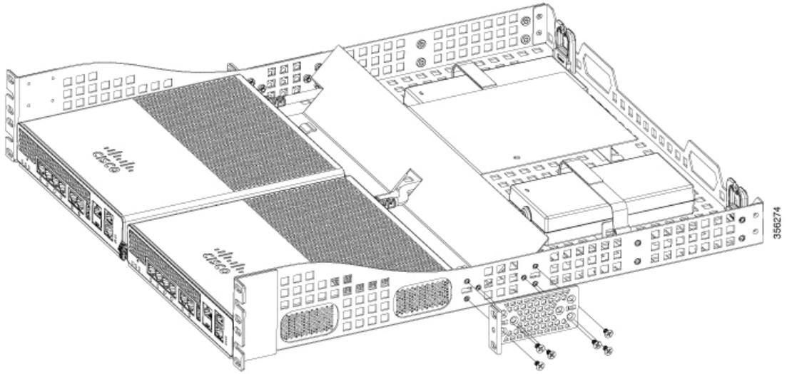
**Note** Install the center mount brackets to both sides of the tray.
