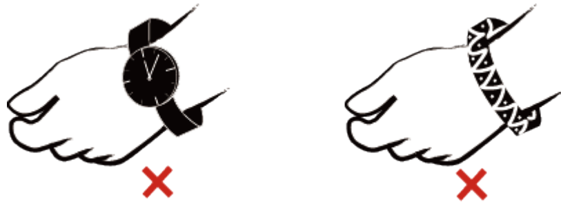
Figure 5-1 Conductive objects to be removed
