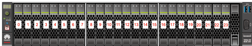
Figure 2-20 Drive numbers of a server with the 24 x 2.5-inch drive pass-through configuration
