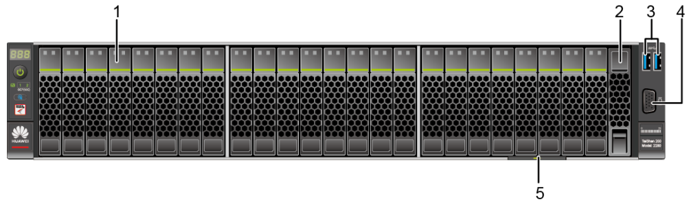
Figure 2-4 Components on the front panel of a server with 24 x 2.5-inch drives
