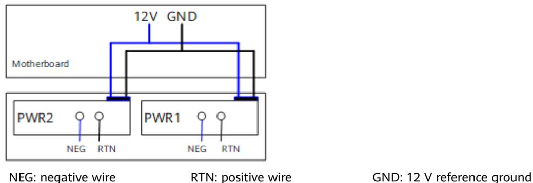
**Figure 4-61** shows the power supply connections of dual AC power modules. After AC power is transmitted to the PWR module, the PWR module provides 12 V output voltage, and the motherboard provides power for the entire device.
