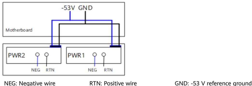
**Figure 4-9** shows the power supply connections of dual AC power modules. After AC power is transmitted to the PWR module, the PWR module provides -53 V output voltage, and the motherboard provides power for the entire device.
