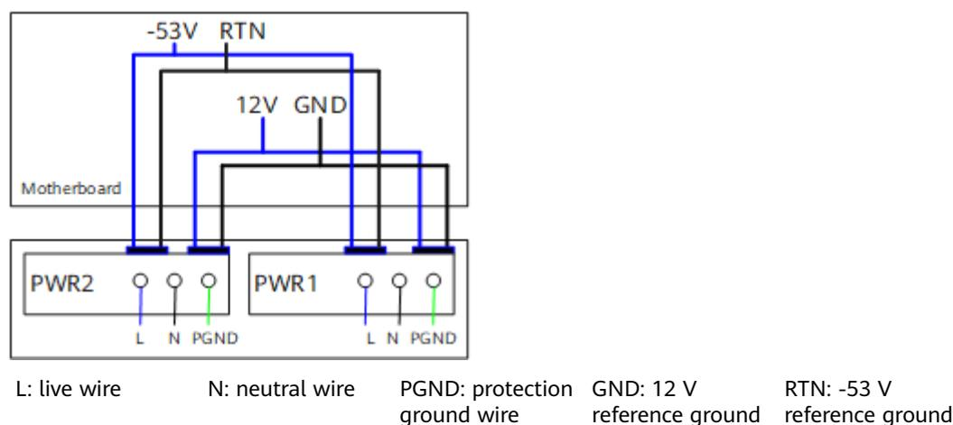
Figure 4-51 shows the power supply connections of dual DC PoE power modules. After DC power is transmitted to the PWR module, the PWR module provides 12 V and -53 V output voltages, and the motherboard provides 12 V voltage for the entire device and -53 V voltage for the PDs.
