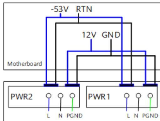
L: live wire      N: neutral wire      PGND: protection ground wire      GND: 12 V reference ground      RTN: -53 V reference ground
