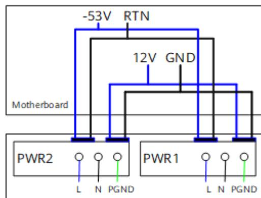
L: live wire      N: neutral wire      PGND: protection ground wire      GND: 12 V reference ground      RTN: -53 V reference ground
