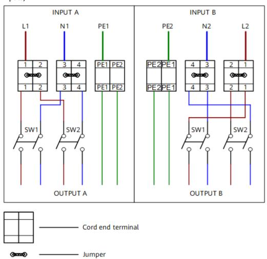
**Figure 5-28** Power distribution in a 2200 W AC power distribution box (two inputs)
