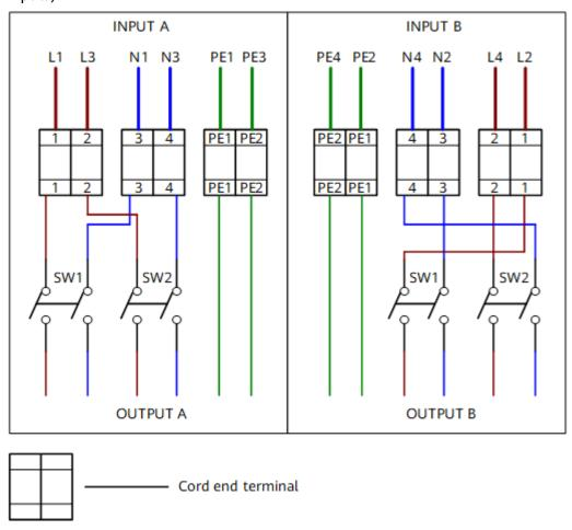
**Figure 5-30** Power distribution in a 2200 W AC power distribution box (four inputs)
