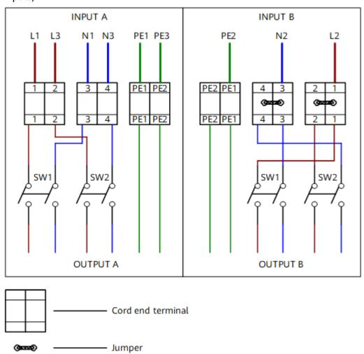
**Figure 5-29** Power distribution in a 2200 W AC power distribution box (three inputs)
