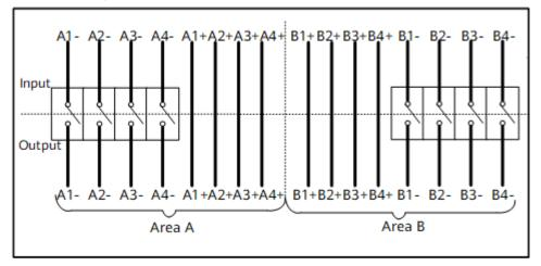
**Figure 5-24** Power distribution in a 2200 W DC power distribution box (four inputs and eight outputs)
