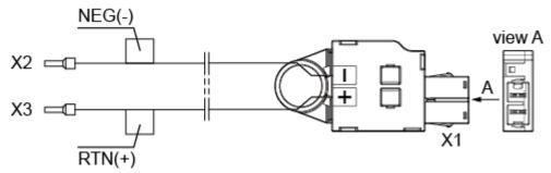
**Figure 8-7** and **Figure 8-8** shows the appearance of the power cable for a 1200 W DC power module.
