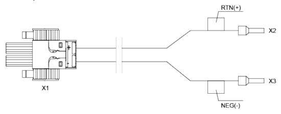
**Figure 8-10** Structure of the power cable for a 1200 W DC power module (nylon insulation terminal)
