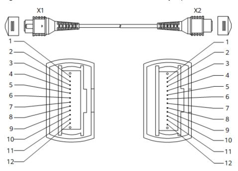
**Table 8-12** Pin assignments of a 12-core MPO-MPO fiber jumper
