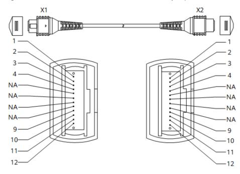
Table 8-11 Pin assignments of an 8-core MPO-MPO fiber jumper
