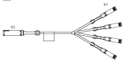
Figure 8-39 Structure of a QSFP-DD to QSFP-DD high-speed cable
