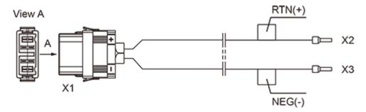
**Figure 8-5** shows the appearance of the power cable for a 1000 W/1200 W DC power module.
