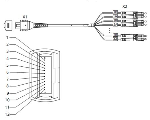
**Table 8-13** Pin assignments of an MPO-4\*DLC fiber jumper
